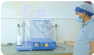
Motorized Denier Test
