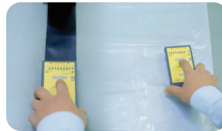
Surface Resistivity Test-Liner
